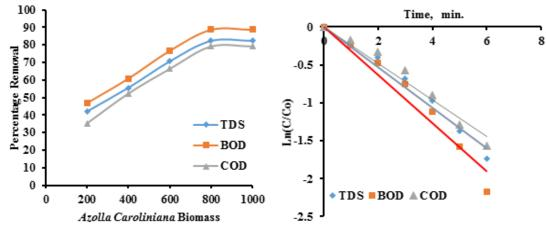
Fig.3.Effect of *Azolla Caroliniana B*iomass on Removal of TDS, BOD and COD from paper mill effluent
